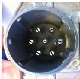
Split-Pins are standard, however solid pins an option
