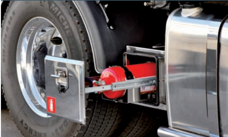
Semi-trailer equipped with pullout BAWER FIRE EXTINGUISHER BOX.
